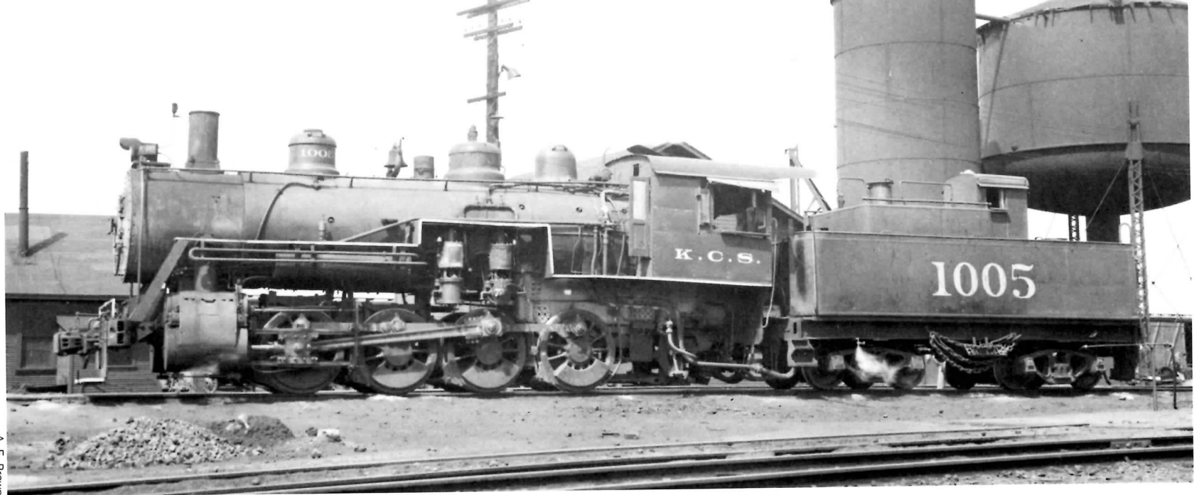
Much-rebuilt Vaucain Compound 2-8-0 469 ultimately became 0-8-0 1005 (above), as seen at Kansas City, Mo., July 2, 1953. K-class 0-8-0 1011 (below), at Pittsburg, Kan., May 30, 1947, was formerly E-2 Consolidation 460, also a Vaucain Compound.
