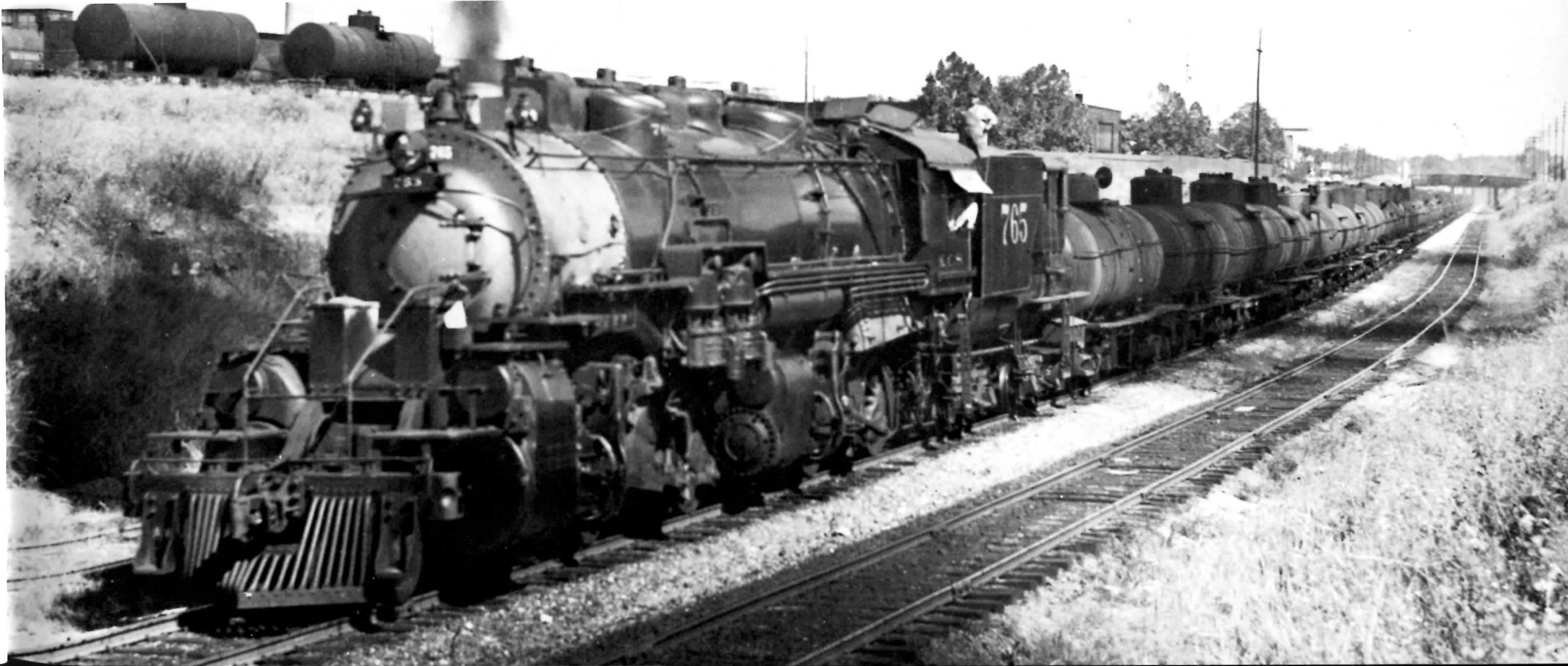
G-2, 757-766, 26&41x32cyl, 57"DR, 250BP, 495,000wgt, 122,600TF(Compound), 147,220TF (Simple), Brooks, 1924
