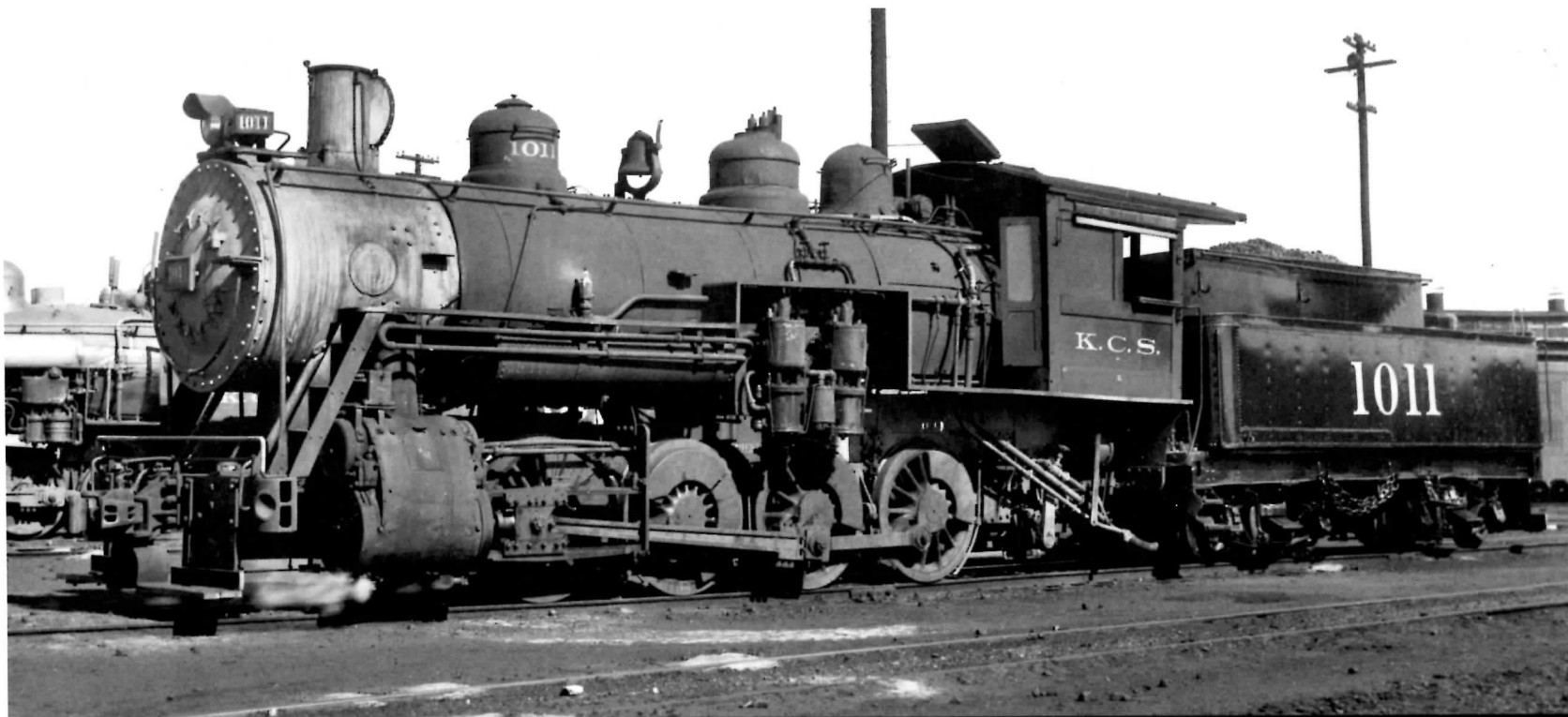
Much-rebuilt Vaucain Compound 2-8-0 469 ultimately became 0-8-0 1005 (above), as seen at Kansas City, Mo., July 2, 1953. K-class 0-8-0 1011 (below), at Pittsburg, Kan., May 30, 1947, was formerly E-2 Consolidation 460, also a Vaucain Compound.
