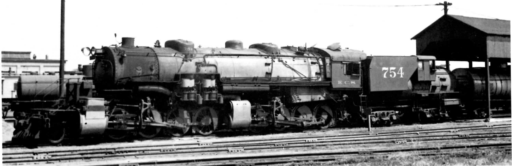
G-1(rebuilt), 750-756, 26&41x32cyl, 57"DR, 250BP, 495,000wgt, 122,600TF(Compound),147,220TF(Simple), Schen., 1918
