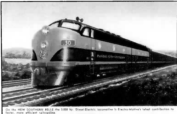
On the NEW SOUTHERN BELLE the 3,000 hp Diesel-Electric locomotive is Electro-Motive's latest contribution to faster, more efficient railroading.
