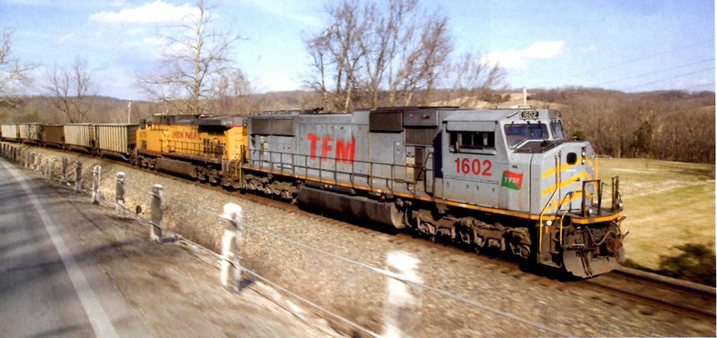
In distributed power mode, a KCSdeM (formerly TFM) SD70MAC and UP AC4400CW team up on a coal empty north of Lanagan, Mo. Chris Guss
