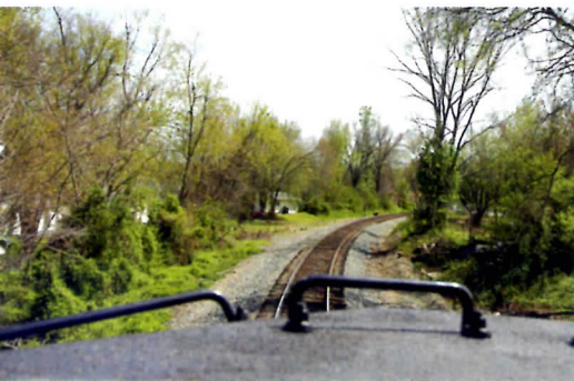
McElhany Hill's 1.5 percent climb is clearly visible from the cab of CKCSH. Fred W. Frailey
