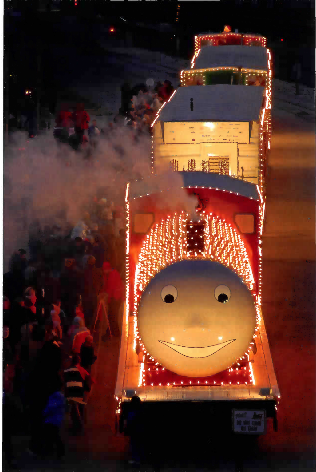
"Rudy" is a makeshift steam locomotive fashioned from a tank car shell and flatcar, with a steel drum for a smokestack. With theatrical smoke and an air whistle hooked up to a compressor, it charms visitors at Kansas City Union Station in 2008. Roy Inman
