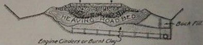
Tile installed under a typical squeeze.
