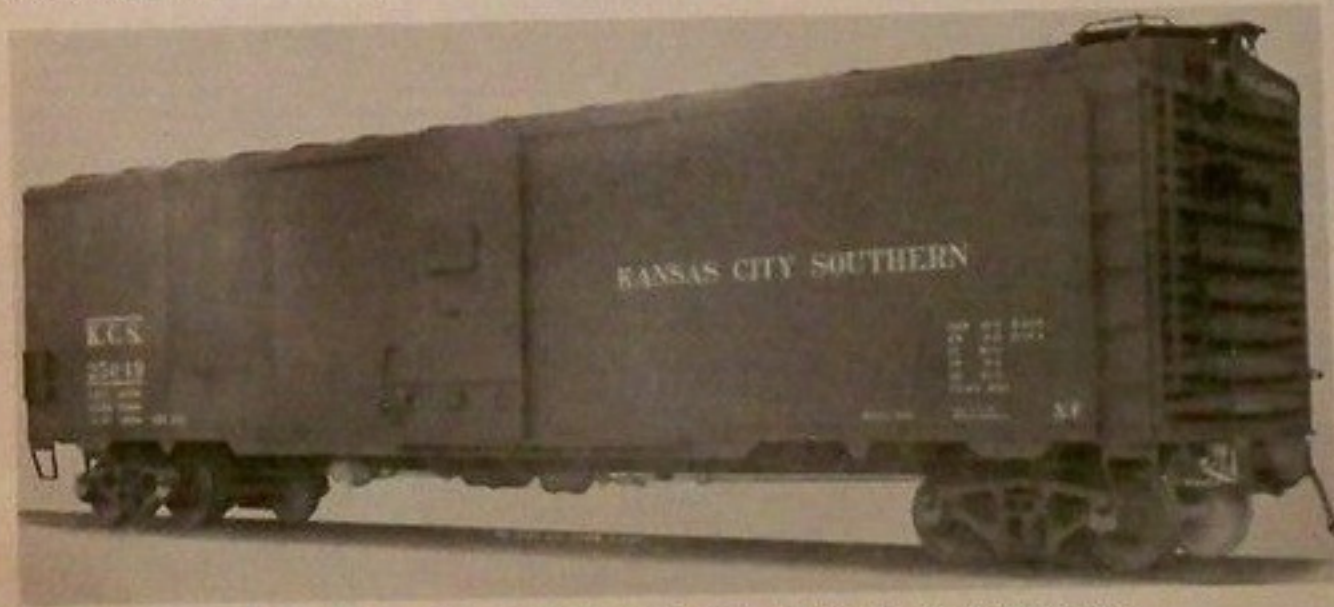
Lightweight Corten Steel Eliminates 9,000 lbs. Weight in this Furniture Car
