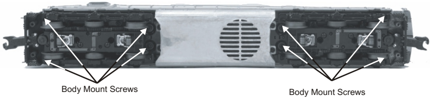
Body Removal Screw Locations
